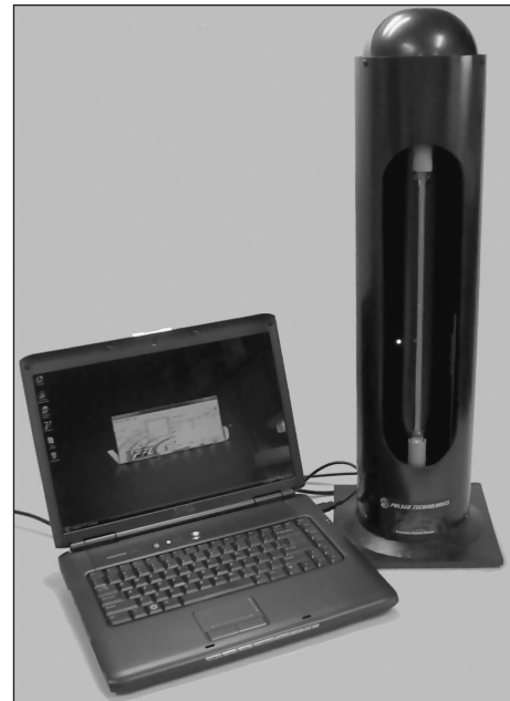
The P3+ (Precision Pulsed Plasma) device. The light tube contains an internal frequency generator, the company's PFG2. The laptop is loaded with the company's software.
